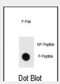
Dot blot analysis of anti-Phospho-MBP-Y203 Antibody (Cat.#AP3556a) on nitrocellulose membrane. 50ng of Phospho-peptide or Non Phospho-peptide per dot were adsorbed. Antibody working concentrations are 0.5ug per ml.
